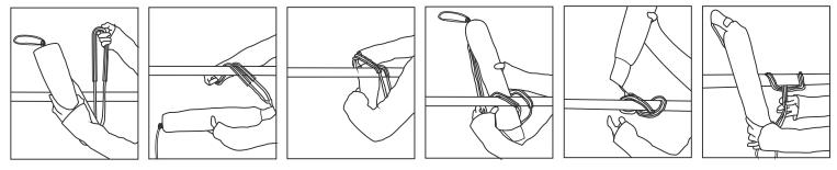
**ATTENTION:** End line is advised to be attached to boat for extra security. Care should be taken when re-packing the retrieval line to ensure successful deployment
