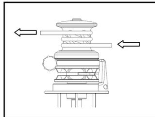
1. Tighten the brake and make sure that the anchor is appropriately blocked.
