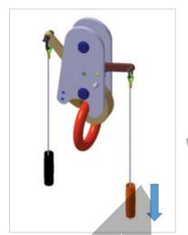
When the liferaft / rescue boat reaches the water, the load on the hook will be reduced and eventually, when the load on the hook is small enough (between 5-30 kg), the hook will open.
